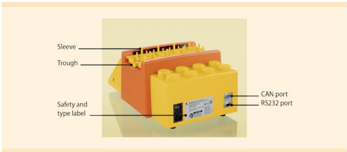
Figure 4.3: Back of the gentleMACS Octo Dissociator with Heaters, Safety Shield removed.
