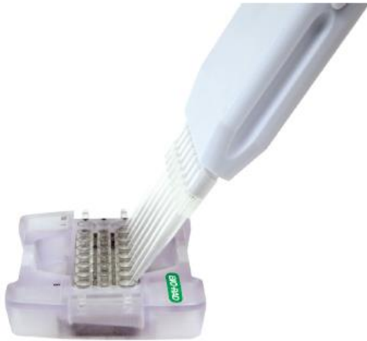
Aspirating droplets from the DG8 cartridge.
