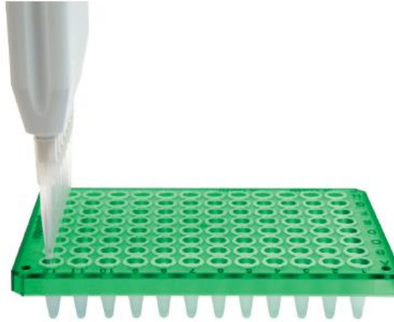
Dispensing droplets into a 96-well PCR plate.
