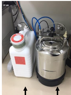
Waste Tank Sheath Tank
